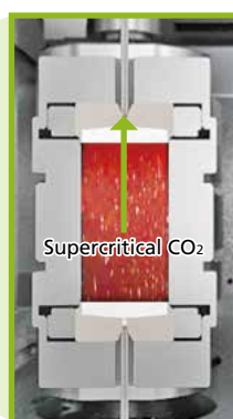
Inside of the extraction vessel encapsulating the sample
