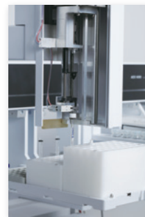
After the analysis is finished, the liner is returned to the tray.
