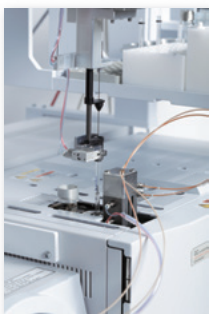
The liner is inserted to the inlet.
