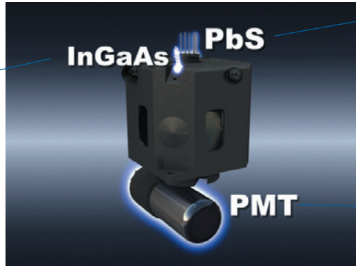
Three detectors attached to the integrating sphere
